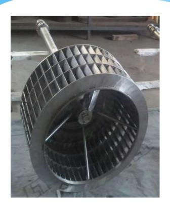
We are manufacture furnace RC Fan in Material SS 304,SS 316 & SS 310 with best Material & best quality.
